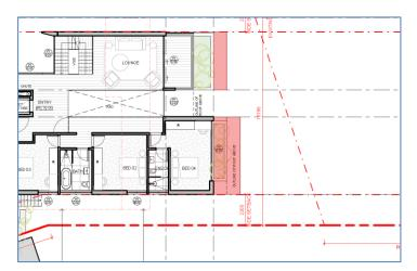
iii. The deletion of the rear roof overhangs at ground floor level and the rear western planter at first floor level as shaded in red in the image below:
