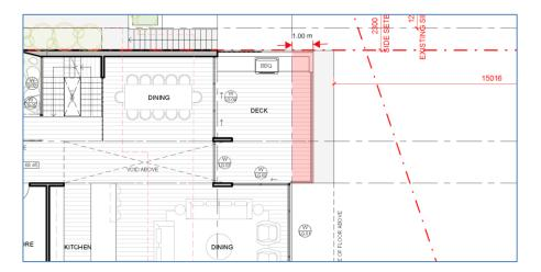
ii. The deletion of the rear roof overhangs at lower ground floor level and the rear western planter at ground floor level as shaded in red in the image below:
