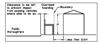
The Principal Contractor or Owner-builder must ensure that overhead protective structures are installed and maintained in accordance with the NSW "Code of Practice - Overhead Protective Structures 1995". This is code available at <a href="https://www.safework.nsw.gov.au/">www.safework.nsw.gov.au/</a> data/assets/pdf file/0008/52883/Overhead-protective-structures-Code-of-practice.pdf
