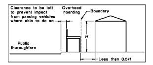
The Principal Contractor or Owner-builder must ensure that overhead protective structures are installed and maintained in accordance with the NSW "Code of Practice - Overhead Protective Structures 1995". This is code available at
