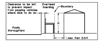
The Principal Contractor or Owner-builder must ensure that overhead protective structures are installed and maintained in accordance with the NSW "Code of Practice - Overhead Protective Structures 1995". This is code available at
