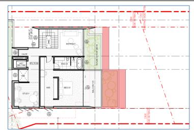
iv. The deletion of the rear roof overhangs at first floor level as shaded in red in the image below:
