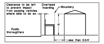
The overhead protective structures must be installed and maintained in accordance with the NSW "Code of Practice - Overhead Protective Structures 1995". This is code available at
