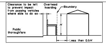
The overhead protective structures must be installed and maintained in accordance with the NSW "Code of Practice - Overhead Protective Structures 1995". This is code available at
