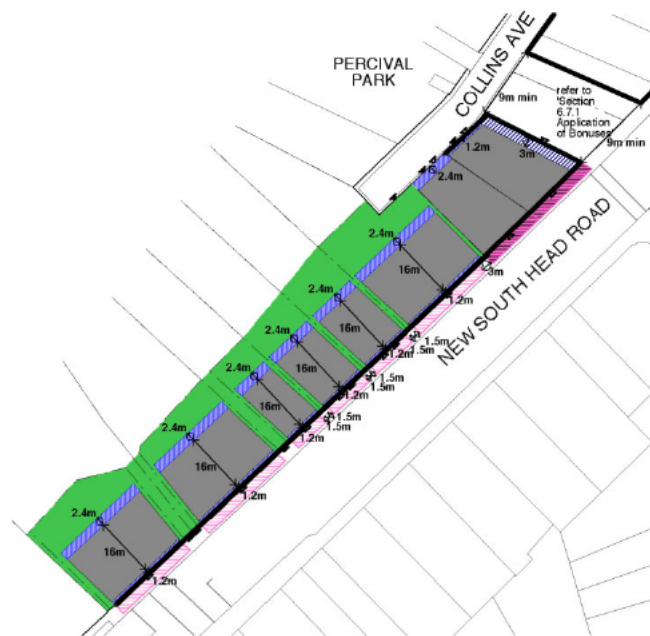
Ground floor level controls
