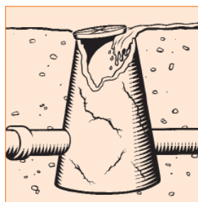
Hidden or damaged maintenance holes
