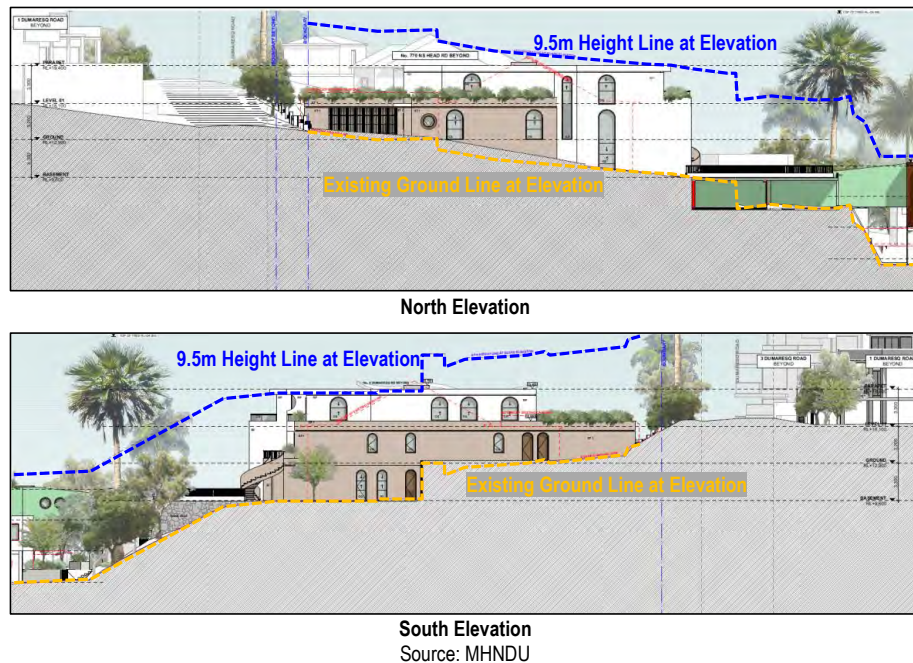
Figure 4: Proposed Side Elevations of the East Wing Showing Apparent Compliance with the 9.5m Building Height Plane
