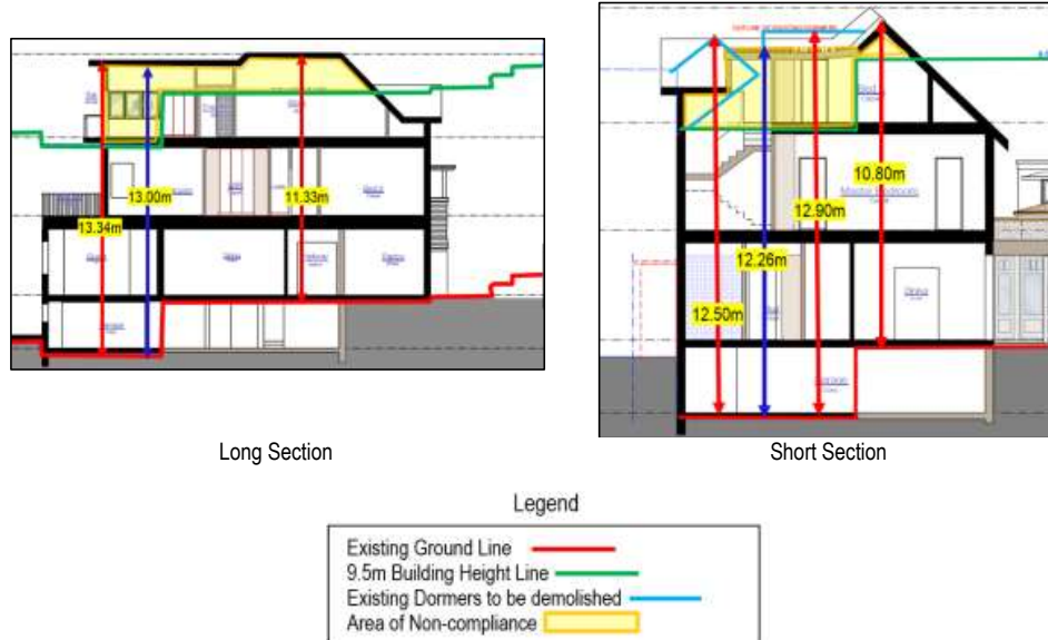
Figure 1: Section Illustrating Maximum Building Height
