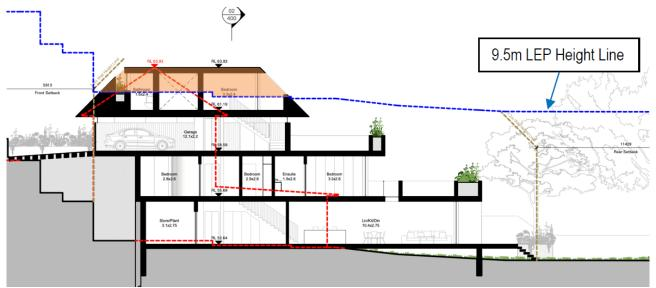
Figure 25: Area of height non-compliance highlighted in orange (Source: Common Office, overlay by Council).
