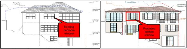
Existing North West Elevation v Proposed North West Elevation (Source: Cave Urban)
