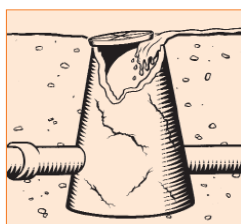
Hidden or damaged maintenance holes
