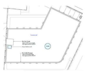
• Mod- DA289/2019/4 for Internal and external modifications was approved on 23/12/2020. External modification works include new air mechanical plenum and relocation of access hatch on the roof (see below extract in blue).
