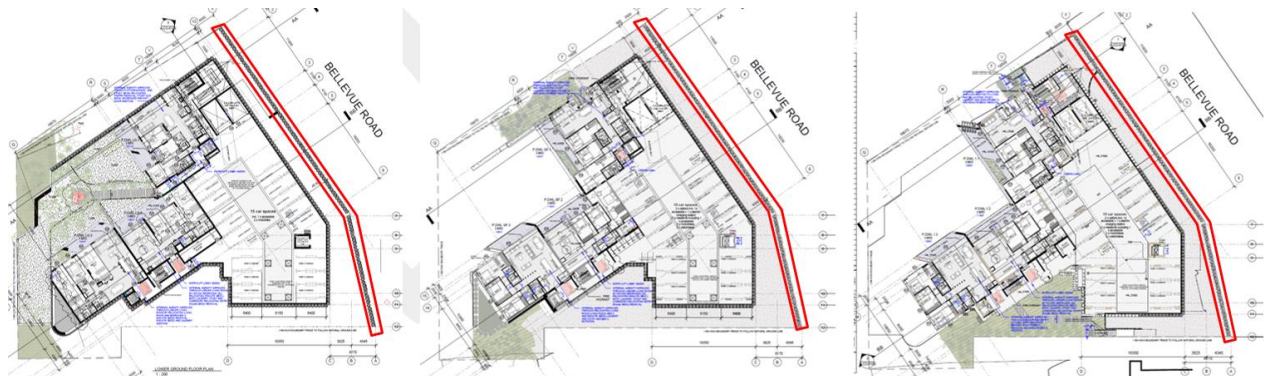
Floor plans of the lower ground floor (left), ground floor (middle) and Level 01 floor (right) showing the contiguous piling running along the entire Bellevue Road boundary of the subject site
