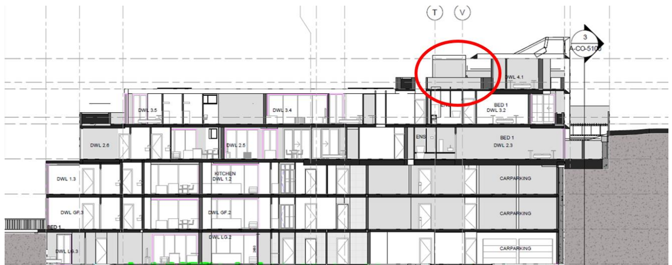
Proposed long section showing the extended lift overrun which appears above the 10.5m LEP Height limit
