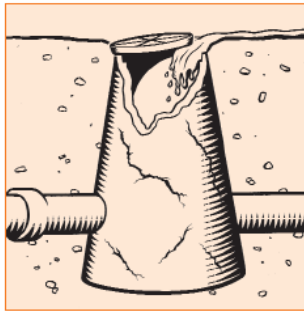
Hidden or damaged maintenance holes
