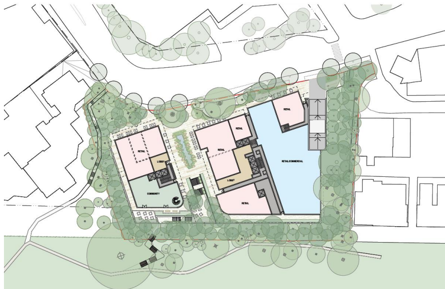
Figure 22 Proposed ground floor plan indicating through site link, commercial floorspace and community facility
