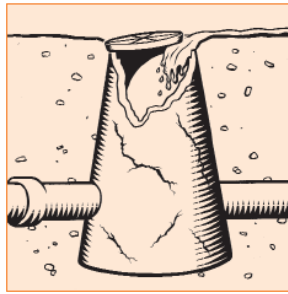
Hidden or damaged maintenance holes
