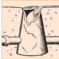
Hidden or damaged maintenance holes
